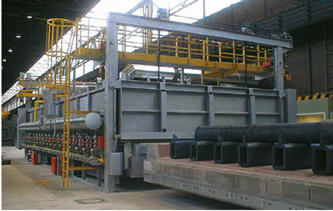
Metallurgical industry: bogie hearth furnace
