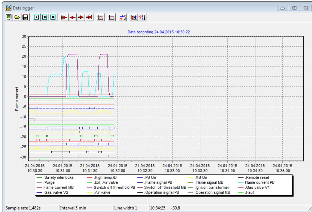
The scanning rate set is displayed in the status bar. The display interval set is indicated beside it.
