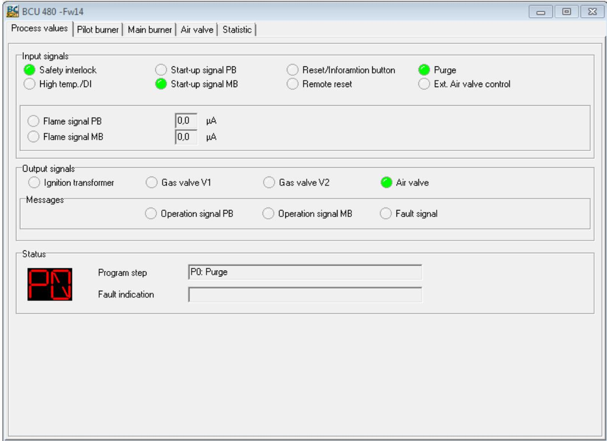
The first time the various tabs are opened, data is read from the device automatically.
