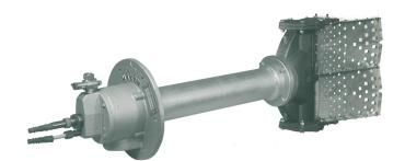
12" back inlet INCINO-PAK<sup>®</sup> burner section shown with (2) LV AIRFLO<sup>®</sup> end plates; includes spark ignitor, pilot gas adjustable orifice, raw gas pilot, and arranged for mounting customer's UV scanner
