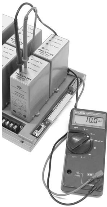
Voltmeter hook-up to a Peek-A-Flame
