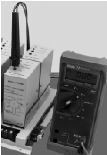
Voltmeter hook-up to a Peek-A-Flame
